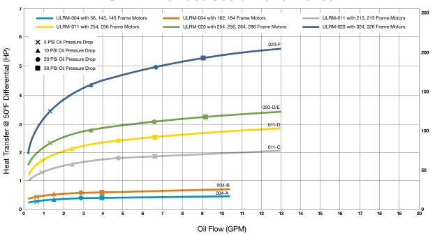
Note: The Cooling capacity curves are based on an Entering Temperature Difference (ETD) of 50°F and ISO VG46 oil.
